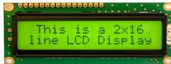
**Gambar. 4 LCD 2x16**
